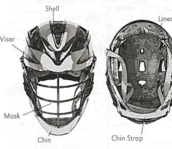
Lacrosse helmets are one of the most expensive and important pieces of equipment. They are made of a plastic shell with an impact-absorbing liner and a metal facemask. Many helmets are custom made to order, so you can select the shell, visor and chin colors at no additional charge.
